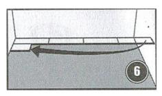
6. Second row First plank min length 500 mm. Put a distance against the wall.
